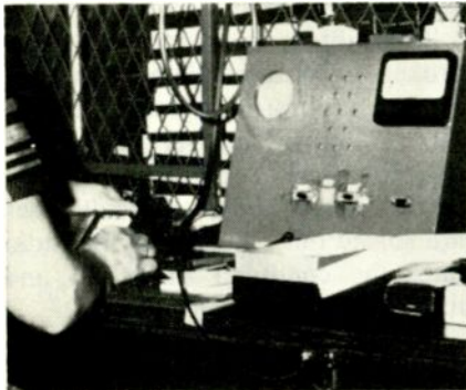
Sensitivity check is final test made before radios are boxed for shipment.
