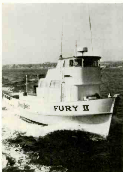
Weather-sealed, 30-in. plastic dome over pilot house contains the 43 lb. radar antenna.
