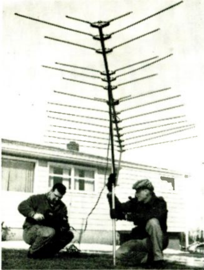
A ground survey using JFD's LPV antenna. This unit proved to be quite effective, though the area where it was installed was a weak signal area.
