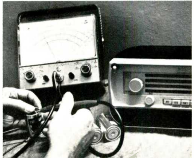
A battery is checked with a VTVM while load resistor is held on battery terminals. Most batteries can be checked in this manner by bending resistor's leads.
