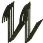
WAVEFORM OBTAINED WITH OPEN TEST LEADS
