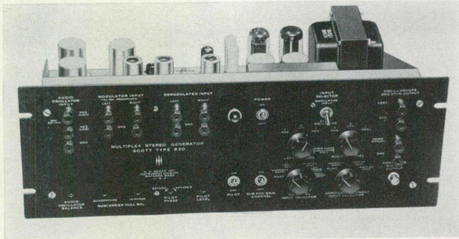
H. H. Scott's Model 830 Multiplex Stereo Generator provides a composite stereo signal. It operates in conjunction with an FM signal generator, audio oscillator and scope.
