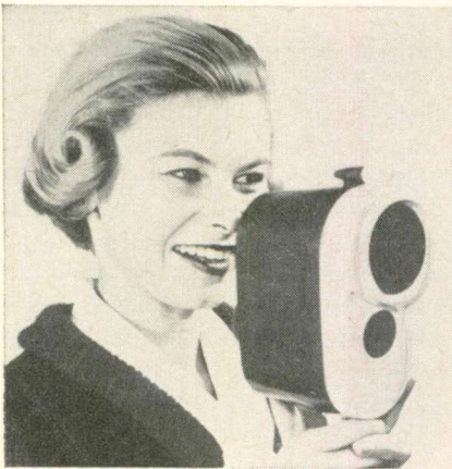
Transistorized wireless two-way telephone-like unit employs sensitive infrared detector.
