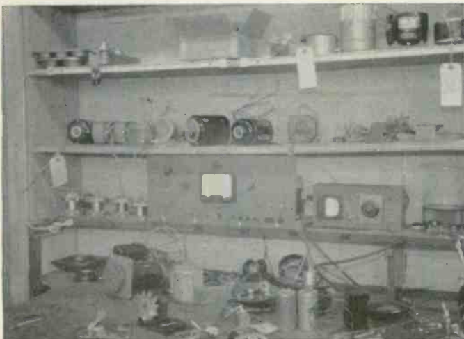
Fig. 5—A motor test and repair bench illustrates the variety of motor types employed in tape equipment.
