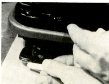
Fig. 2—Chalk marks on record player mounting pins can be transferred to a brown paper or cardboard template to be used for accurately cutting equipment mounting bases.
