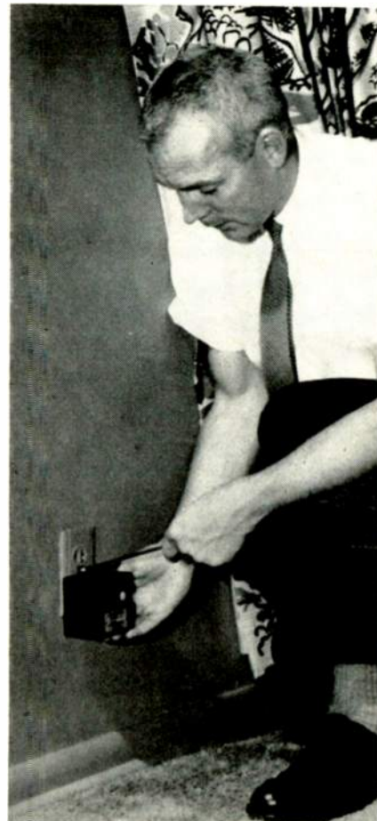
Fig. 1—The NEAR system receiver plugs into a standard double wall outlet just like a lamp. Manufactured at the AC Spark Plug Div. plant in Flint, Mich., it emits a loud warning buzz when activated.
