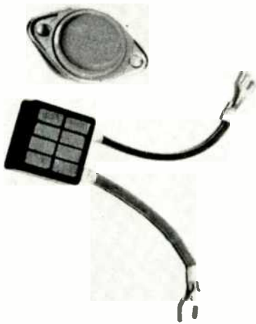
Fig. 1—Frigistor module consisting of eight Neelium thermocouples compared in size with a typical germanium transistor.
