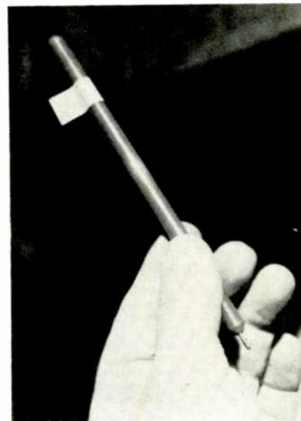
Fig. 2—A color coded pressure-tape "flag" attached to alignment tools, prevents their rolling from bench top. Locating tools is simplified in cluttered surroundings.
