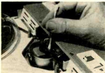
Fig. 1—Q-tips are used to clean delicate tape recorder heads.
