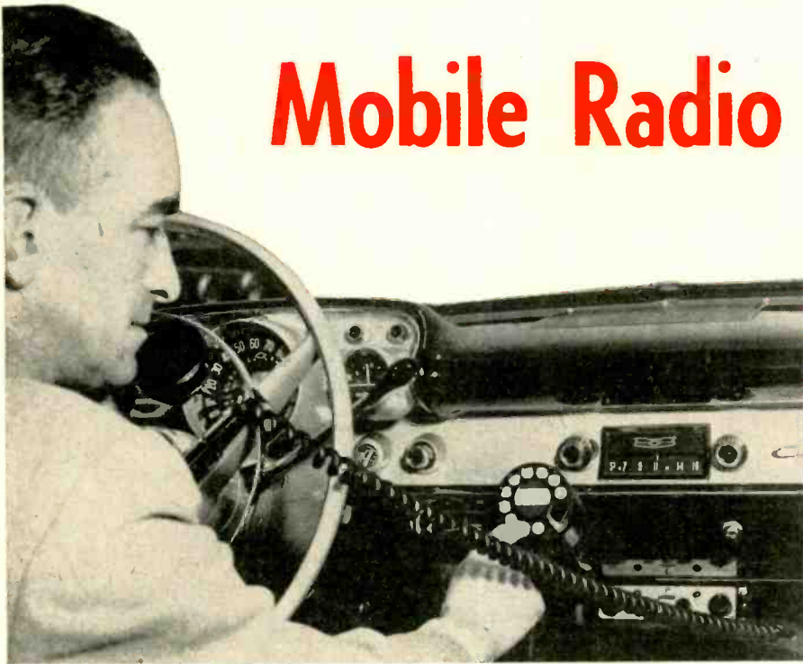
A mobile radio unit equipped with a dial-type selective calling system provides the convenience of private signaling.
