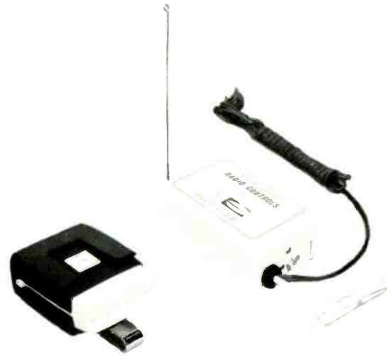
Fig. 1 — Typical VHF solid-state garage door opener transmitter and receiver.
