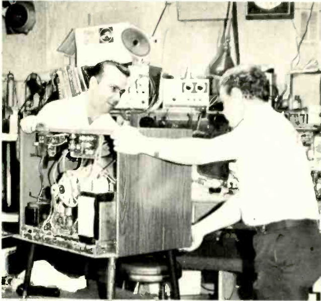
Technicians mount a color TV on portable table for servicing. Table is innovation of technicians and consists of cloth covered bench with legs and casters.
