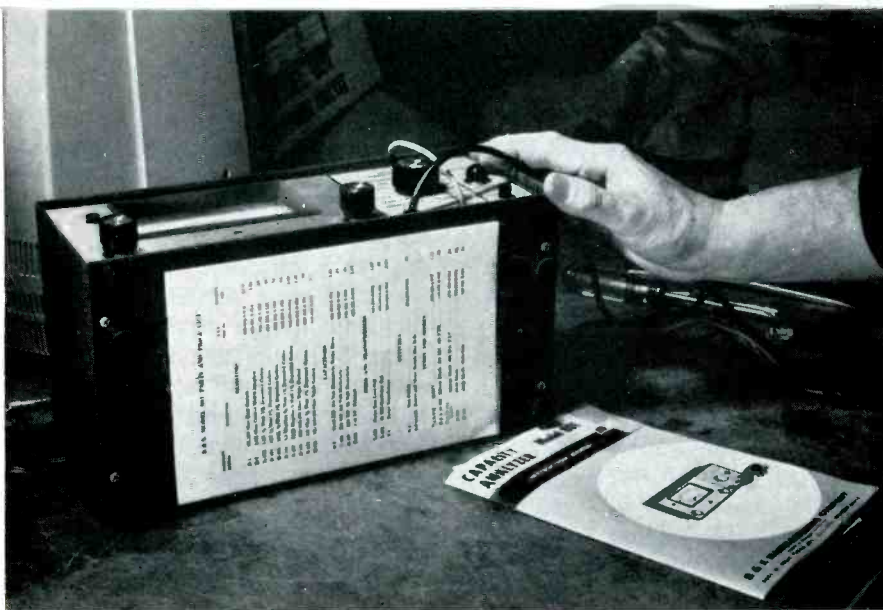
Fig. 2—Important information may be taped to the bottom of a test instrument for safe keeping.
