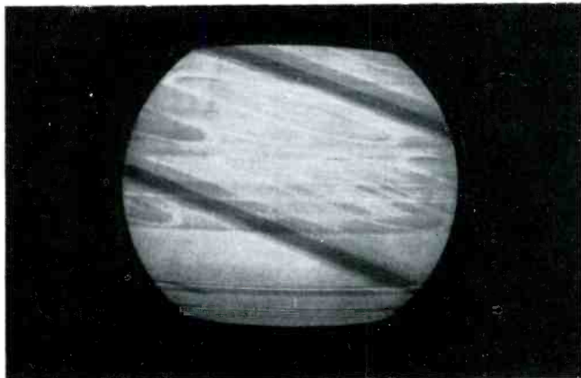
Fig. 5—Out-of-sync, washed-out picture from RCA CTC16 color chassis.
