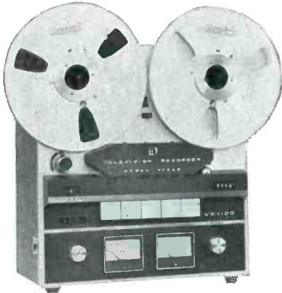
The 1/4 in. tape on AKAI Electric's longitudinal video tape recorder passes the recording head at 30ips.
