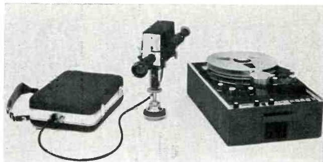
The Westel color-compatible TV recorder (right) plays back tapes from the TV tape camera.
