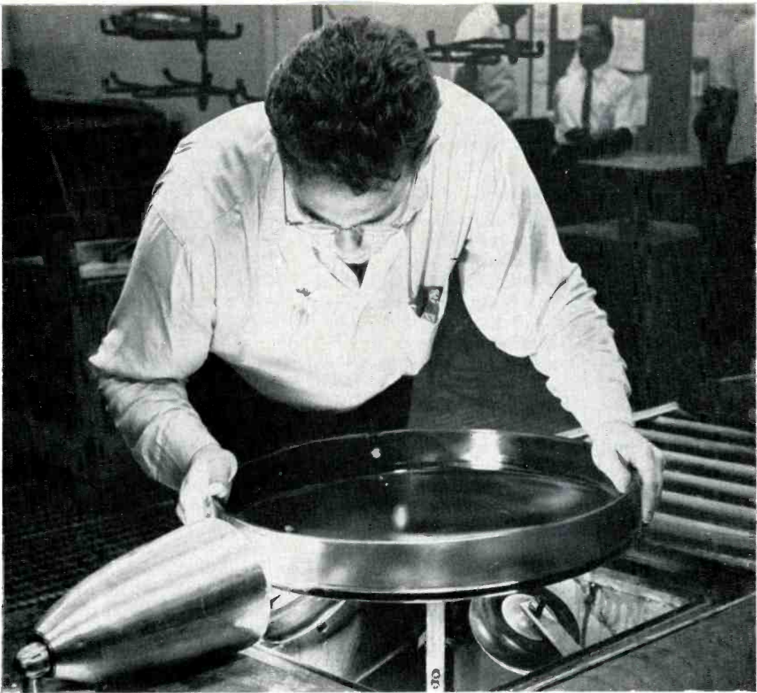
A color CRT faceplate goes through one of a series of inspection steps at the Muncie, Ind., plant of Owens-Illinois, Inc.
