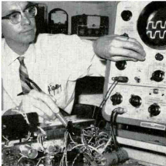
Fig. 4—A 0.003µf capacitor showed loss of gain in one channel as shown on top trace.
