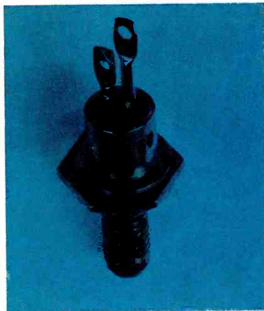
Because of its industrial applications, silicon controlled rectifiers are important semiconductor components.
