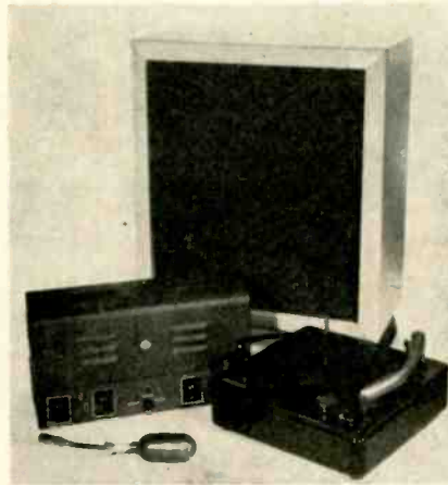
Fig. 3—Elementary system consisting of dynamic mike, 3-speed changer, 15-watt amplifier, and wide-range speaker-enclosure.
