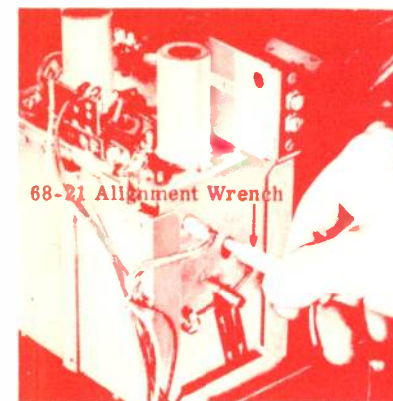
Fig. 11 Bulls-eye Tuning Adjustment.
