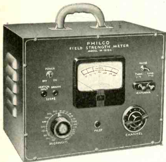
Field Strength Meter
