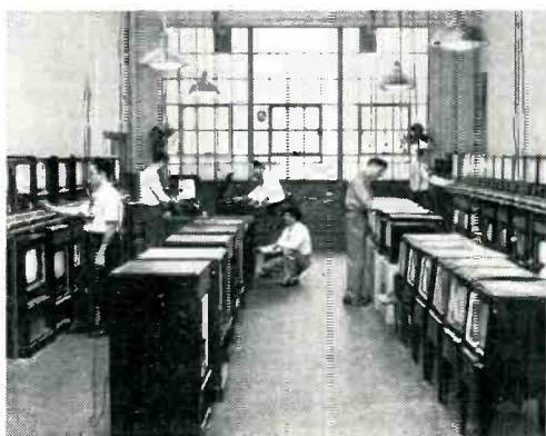
From Each Day's Production, forty completed television sets, packed exactly as a dealer receives them, are selected at random and given a rigorous 40 hour continuous test to assure that every standard of Philco quality is achieved in production.
