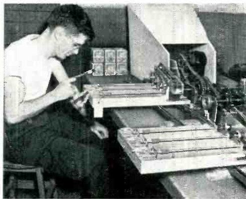
Life Tests. All components of Philco receivers are rigorously life-tested to assure that they meet Philco standards of dependability with an ample safety margin. Here the Philco electronic built-in aerials and television tuners are being tested.
