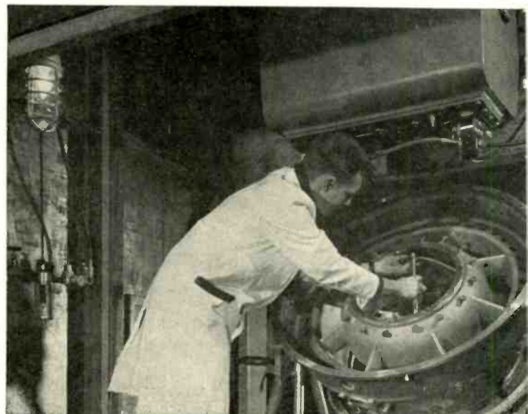
Fig. 3—A self-contained industrial radiographic machine is used here to look for material defects in aircraft engine parts.
