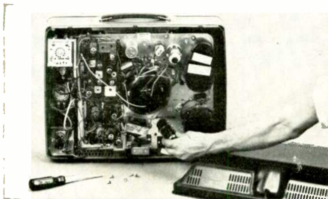
1. 98% OF ALL SERVICE can be done from rear of set with back cover removed! All fuses, tubes and most other parts are easy to reach. No need to remove the chassis.
