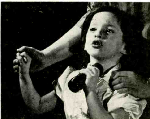
More than 40,000 voiceless people can speak again with the Electro-Larynx developed by Gilbert Wright and Kett Engineering. The portable instrument is held against the throat to vibrate a column of air in the esophagus. By lip, tongue and mouth motions, the sound is modulated into intelligible speech.
