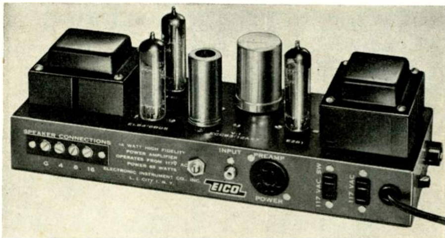
Fig. 1—Hum currents in the transformer laminations also circulate through the chassis. The chassis acts like another lamination. Interaction between transformers can be minimized by wide spacing, and rotation. Transformers having small flux densities and proper shields induce minimum hum.
