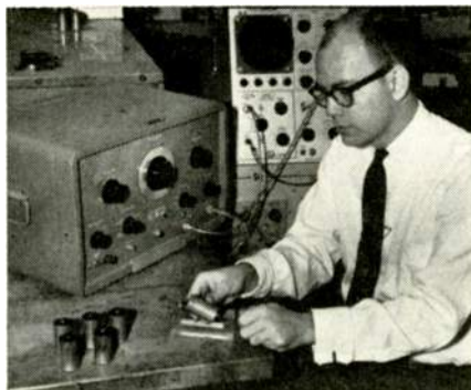
Fig. 1—Measuring the internal resistance of dry cells with a non-destructive pulse method. In the foreground is the cell holder, at left is a pulse generator.
