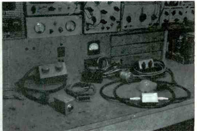
Fig. 2—Assorted mockups for troubleshooting different 2-way radios.
