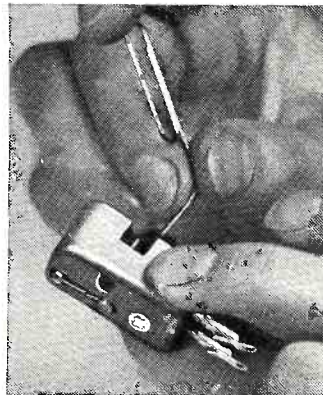
1 Simply remove cartridge from tone arm.
