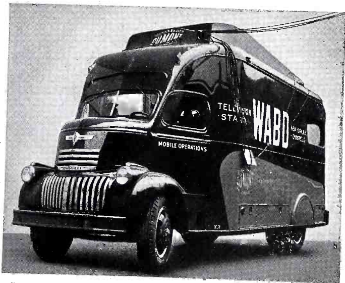
Du Mont's mobile units pick up action wherever it occurs and relay it back to the transmitter.
