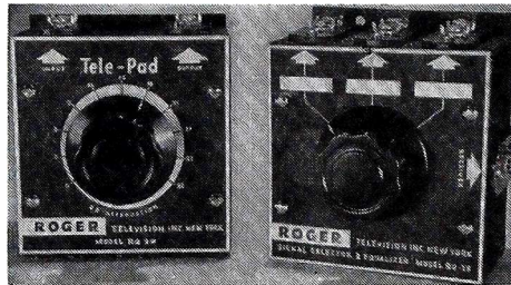
Fig. 3. Left, commercially-available variable pad box. A servicers' instrument, it gives values for set's permanent pad box such as shown at right. Made by Roger Television, Inc., 366 Madison Ave., N. Y., for 300 ohm lines.
