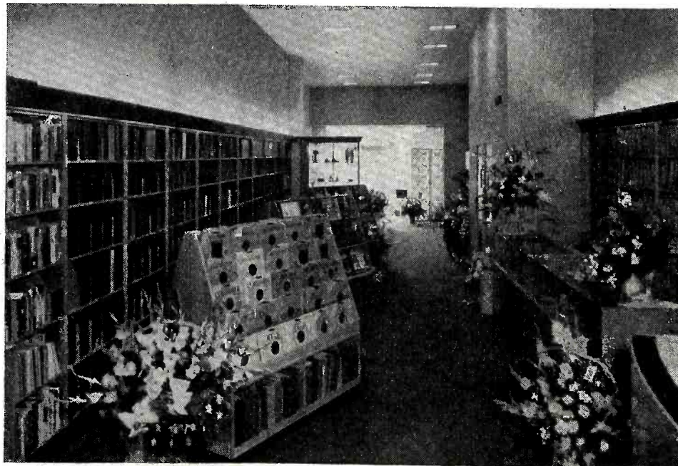
A. Bitter Construction Co., 721 E. 133 St., New York City, completed this new display installation at the Shackleton Piano Co., Louisville, Ky. The fixtures were built in New York, and shipped to Louisville in sectional units. The fixtures are of modern design, and employ selected straight grained Oak in a pickled antique finish. The set-up combines beauty with straight selling efficiency. Note ample storage space and compactness of design. Illusion of spaciousness is carried out, and self-selection encouraged by this floor layout.
