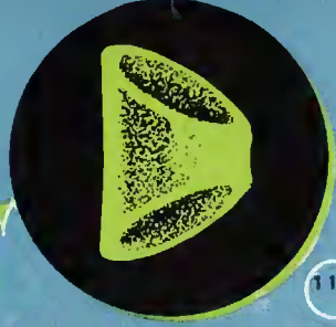
SIMILAR TO 10 (at left) BUT WITH A PHASE SHIFT SHOWING IN AUDIO SYSTEM.
