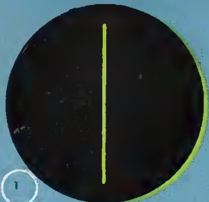
1 USED AS VACUUM-TUBE VOLTMETER. READS PEAK VOLTS AT ANY FREQUENCY.
