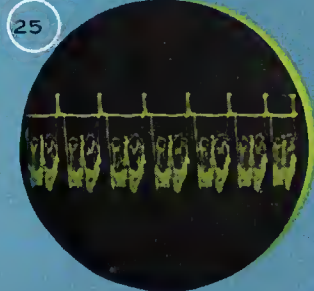
26 SURGE VOLTAGES. TRANSIENTS APPEARING ON HIGH VOLTAGE TRANSMISSION LINE.
