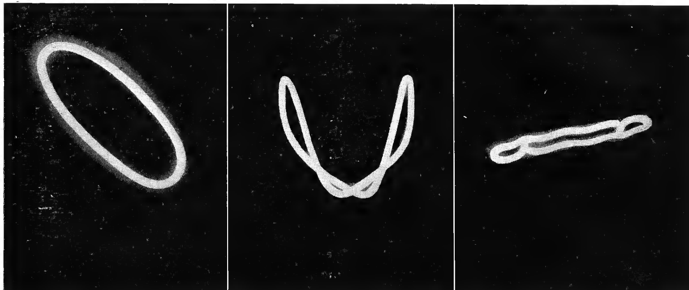
Fig. 5—Hum pattern on left is due to 60-cycle leakage from heater to cathode. Other two patterns show 120-cycle power supply ripple. Pattern at right is about normal for hum in plate circuit of last audio tube.
