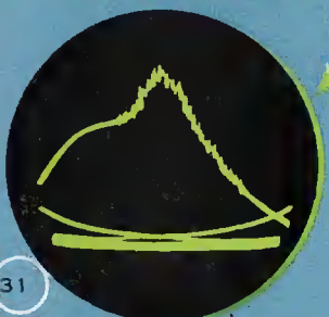
32 FIRING STRESSES IN GUN BARRELS CAN BE DELINEATED USING STRAIN-GAGES.
