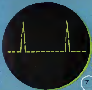
BALLISTIC STUDIES. BEAM MODULATION OR "Z" AXIS GIVES TIME DOTS ON LINES.
