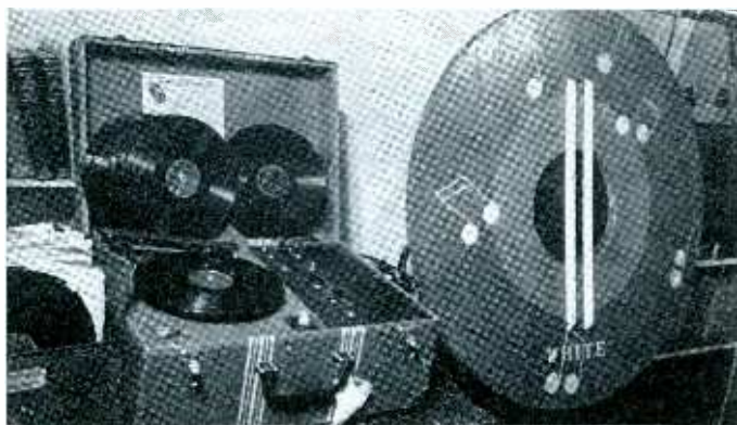
EQUIPMENT FOR LARGE AFFAIRS—Portable case houses amplifier and motor. External speaker mounted on 36 inch circular baffle. Thirty dance records supplied with installation
