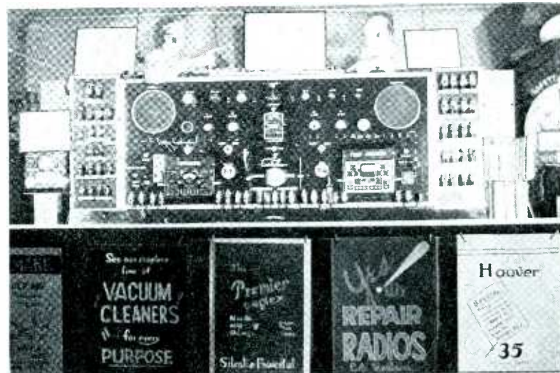
UNIVERSAL SERVICE—Test bench of C. H. Woolley and Son, Inc., Jamaica, N. Y., boasts complete facilities for testing radio and sound equipment. Note the handy selection of tubes which is convenient for the servicer and impressive to the customer
