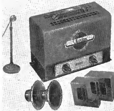
SOUND SYSTEM—Model C-410, popular size sound system. Uses 6V6G pushpull beam power output tubes; supplies 10-15 watts of audio; phono and mike input; speaker matching transformer; complete with 2 speakers, baffles, microphone and stand, $76.47 list. Transformer Corp. of America, 69 Wooster St., New York.
