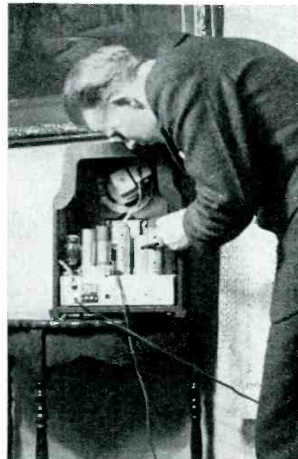
Having obtained a few pointers, check through each stage by tapping tubes, connections and parts carefully
