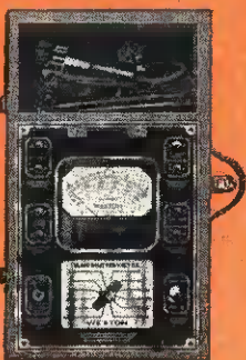
WESTON Model 772 Super Sensitive Analyzer
