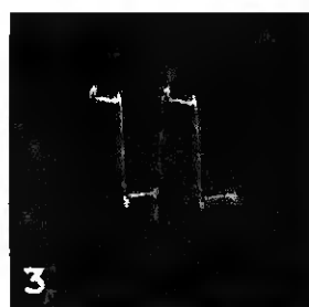
Vibrator at approximate end of life. Ragged edges in horizontal trace mean pitted contacts (3). Single-footing vibrator (4) due to worn contacts or low supply voltage.
