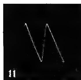
Half-wave rectifier shows ripple curve like (11) across input filter. With vertical gain increased output ripple is as in (12).
