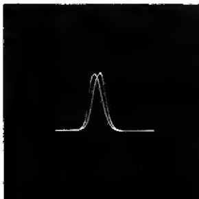
5 TWO STAGES—Last stage correctly aligned, first stage misaligned (5). Both stages aligned (6). Resonant peak sharper than single unit in (2).
