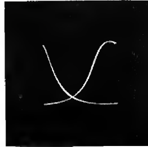
3 WRONG TIMING—Last stage correctly tuned but with time-axis-oscillator set at twice correct frequency (3); one-half correct frequency (4).
