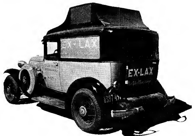
An ingenious method of inclosing trumpets devised by Radio Research Laboratories. The equipment is "streamlined" into the top.
