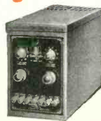
The Sentinel B-C Power Unit furnishes both B and C voltage for any set, regardless of the number of tubes—80 mil. at 180 volts. Price $44.50
