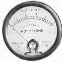
Dial showing double scale for filament and battery voltages.
