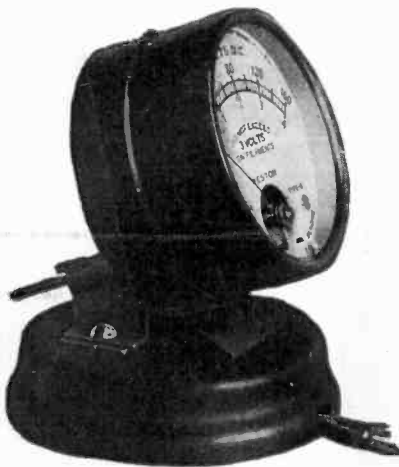
Testing "B" Battery with the Pin-Jack Voltmeter and High Range Stand.
