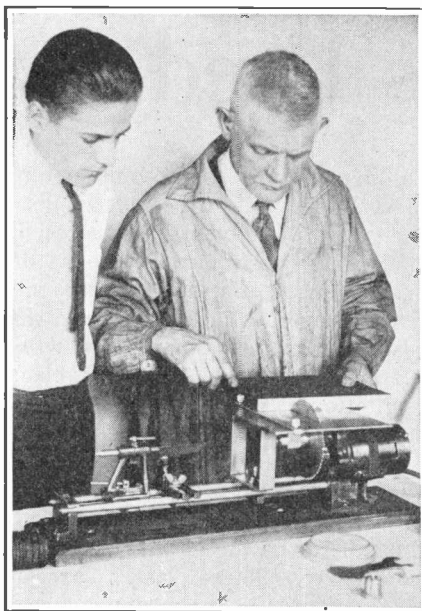
Speeding up service as well as profit can be done by the above illustrated portable shop. This is made by the Electro-Magnetic Tool Company, Cicero, Ill. The service man is here shown cutting a piece of bakelite which is but one of the many things that can be accomplished on this machine.
