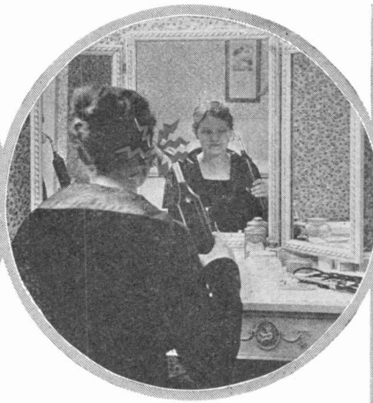
One of the worst producers of "local interference," the violet-ray outfit, can also be remedied by condensers.
