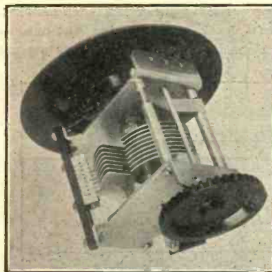
Fig. 5. A View of a Condenser Which Shows no Crowding of High Frequency Stations
