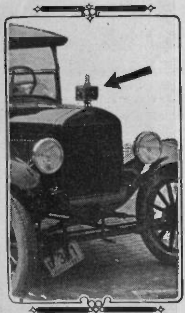
The arrow points to one of the smallest factory-built radio sets. It is the one-tube Crosley "pup," only 3¼ inches high. Its size may be compared with the radiator of the new Ford.
