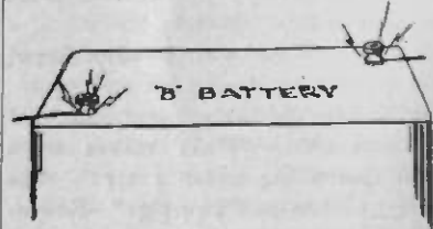
Fig. 6. Poor Battery Contacts May Be Hidden Under the Wax Top
