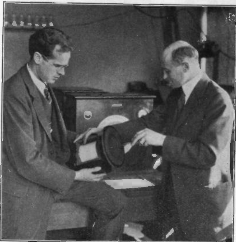
Fig. 7. The Rubber Baffle Around the Edge of Diaphragm is Seen in This Picture.
