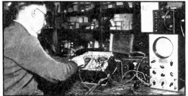
Figure 3 Checking set with an oscilloscope. Note the layout of receiver, oscillator and oscilloscope.
