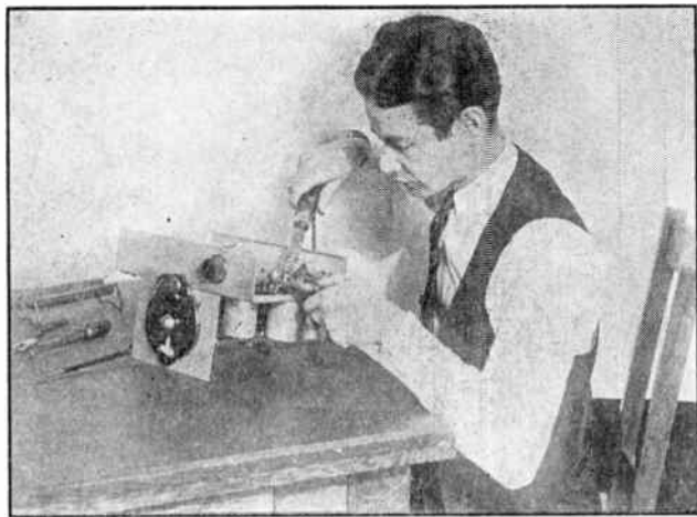
Figure 70 shows how A.V.C. is added to the receiver. A half hour's work and the t.r.f. receiver is provided with automatic volume (sensitivity) control.
