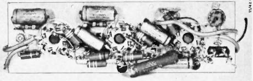
The amplifier section was constructed on an "L"-shaped aluminum bracket with shield.
