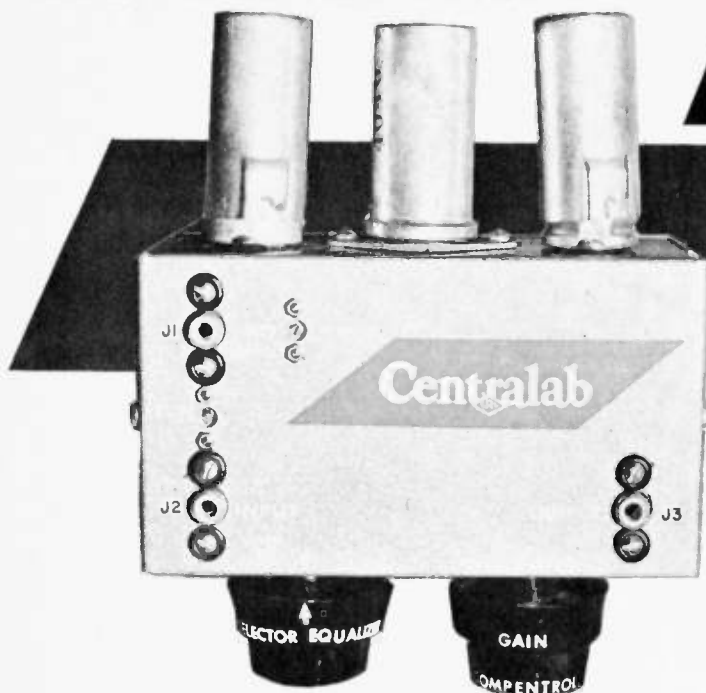
Fig. 1. The Printed Electronic Circuit preamp which measures 5½"x3"x2½". With equalizers using standard components, the over-all size of the unit will have to be enlarged.
