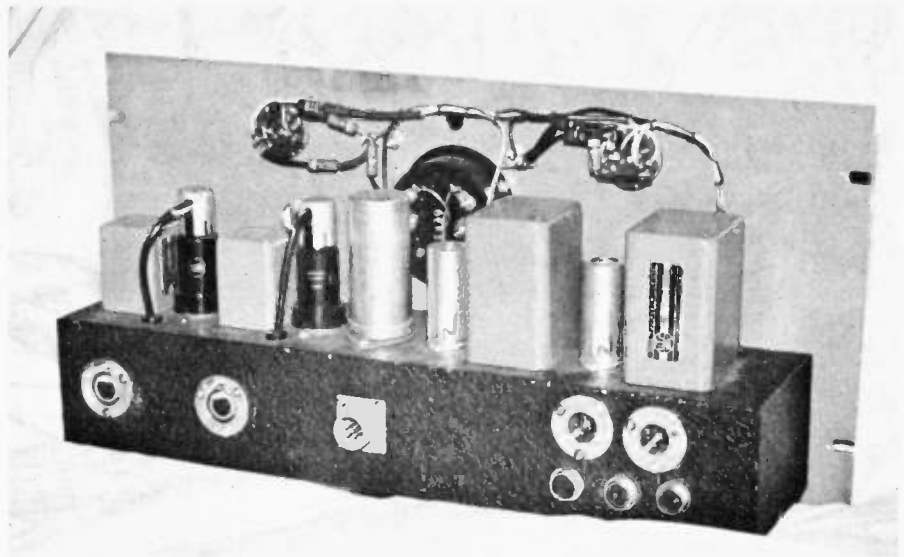
Rear view of unit. Note particularly the type of jacks and plugs that were used in the construction of this unit. It is important that all of these components be of the shielded type to prevent hum pickup. The jacks and plugs are, from left to right: Mic. 1, Mic. 2, power cable connector, (far right, top) 50 and 500 ohm outputs, (far right, bottom) Phono 1, Phono 2, and tape playback inputs.
