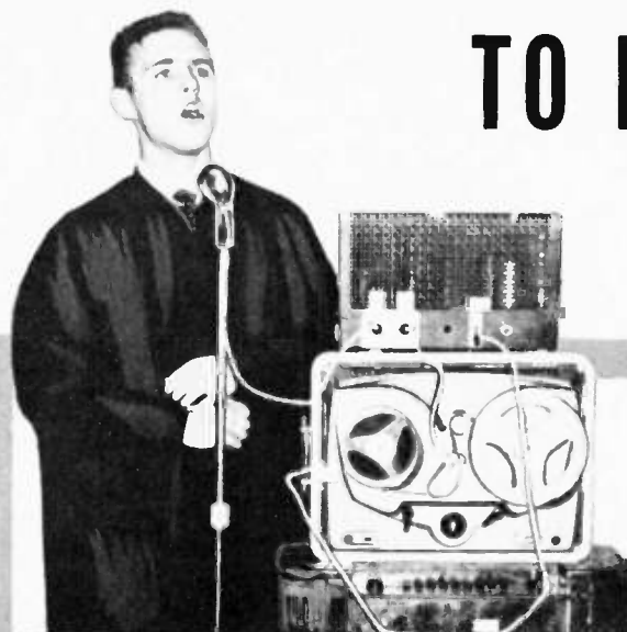
Fig. 1. The actual wiring has been replaced by white cords for purposes of illustration. Additional pickup is seen above regular heads. Steel spring under a head mounting bolt holds the extra head in place. See article.
