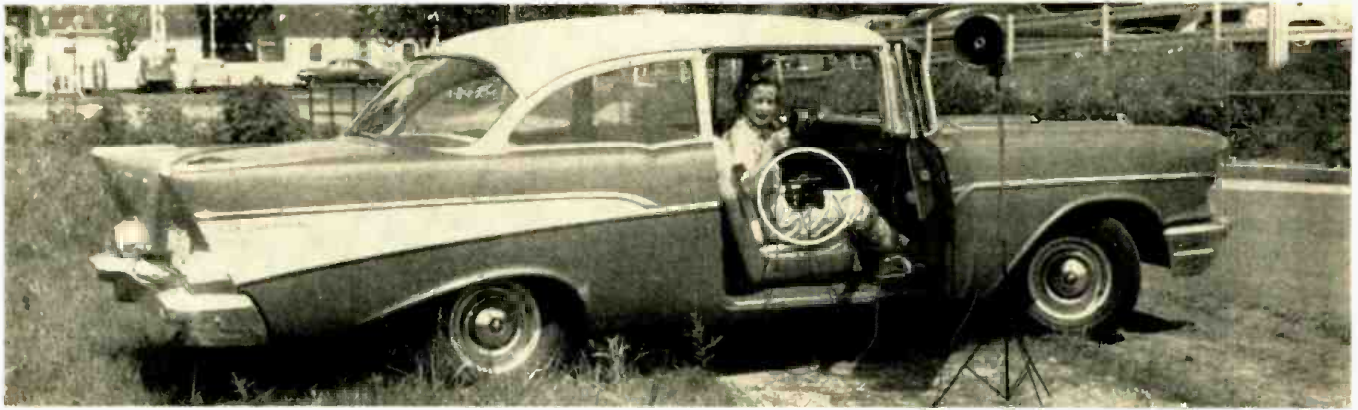
Using "Tiny Tim" with a 25-watt horn type loudspeaker for outdoor activities. The amplifier is held on the lap and is plugged into the cigarette lighter socket.
