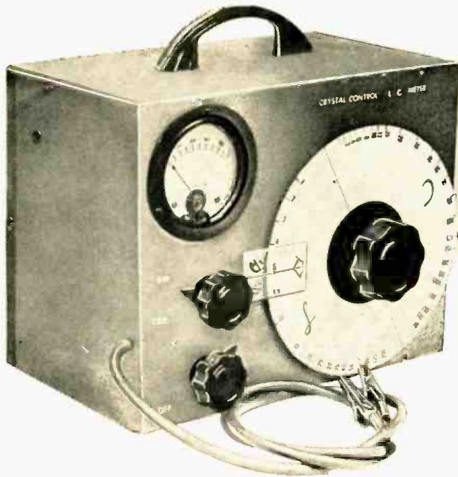
Fig. 1. Dial of the unit is calibrated in units of capacitance and inductance.
