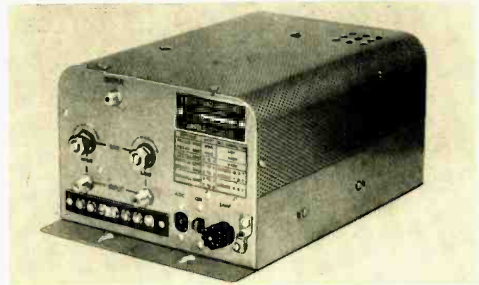
Jerrod 2300 amplifier provides adjustable gain and tilt.
