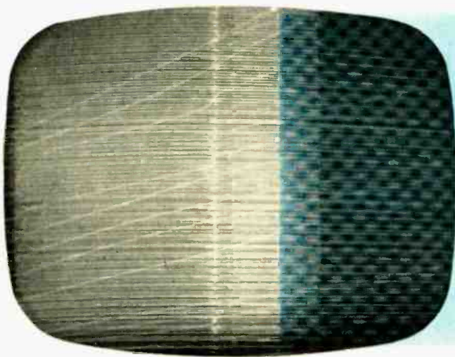
Fig. 1. In this puzzling intermittent, the raster would occasionally break into a "Christmas-tree" pattern, as shown. The cause was run down by taking voltage readings in the horizontal oscillator stage with the tube out of its socket.
