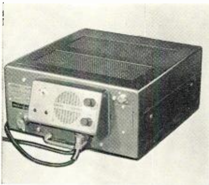
General Electric's desk-top Citizens Radio station is housed in a mobile-type case that will front-mount under auto dashboards or under truck seats.
