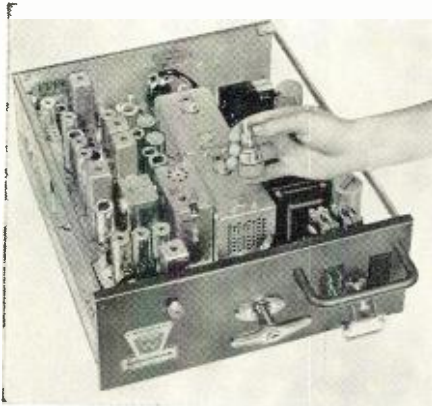
Motorola's mobile unit has an r.f. power output of over 18 w. and uses two 2C39A's in tuned cavity circuits as tripler-driver and final amplifier.
