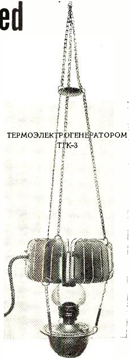
The "Thermo-electro Generator TKG-3" not only supplies heat and light but may also be used to cook some borsch in a pan placed atop the radiating fins. The wire lead from the built-in thermocouple is shown.
