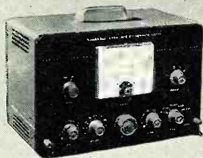
HARMONIC DISTORTION METER
