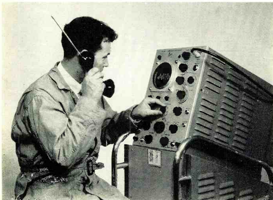
George Bryan demonstrates an experimental model voice-operated radio transmitter at the Signal Corps Engineering Laboratory. The impact of the sound waves from a speaker's voice powers the electronic signal. Jobs involving interesting new equipment such as this transmitter are open in various branches of government service.
