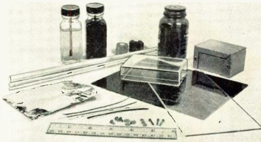
Fig. 3. "Accessory" items used in assembling small equipment. Service cement, Bakelite cement, Scotch tapes, aluminum and plastic boxes, foil, tubing, etc. are shown.
