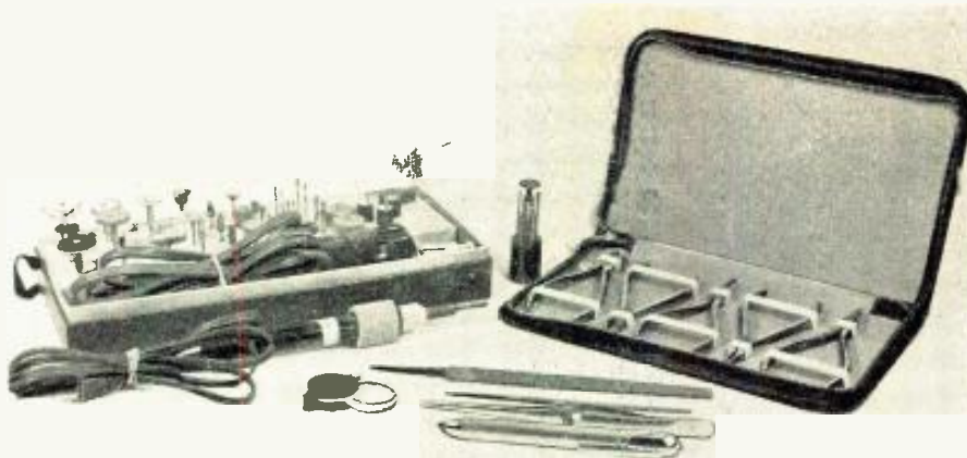
Fig. 2. Some of the tools that the builder of subminiature gear will find useful. Shown are power tool, jeweler's screwdrivers and pliers, soldering pencil, etc.
