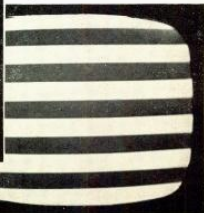
Fig. 5C. Injected at the converter plate, test point 8, the AM i.f. signal shows deepest contrast, evidence of greatest gain in normal operation.
