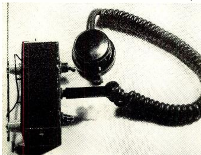
Over-all view of the "transmitter." In this case, antenna is mounted on case with stand-offs. Mike is a surplus T-17 unit.
