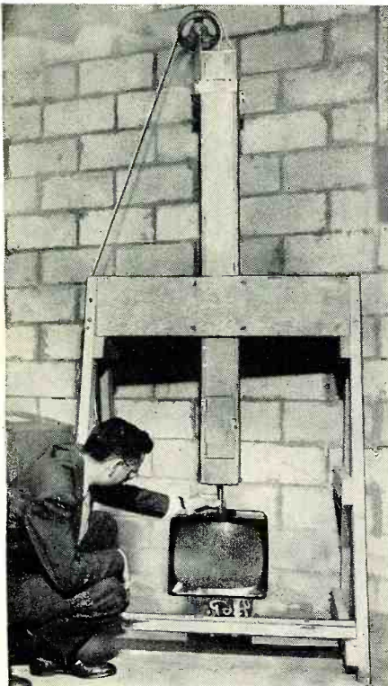
Fig. 1. This "guillotine" drops a weight upon the picture tube through a hole in cabinet. This causes the CRT to implode.
