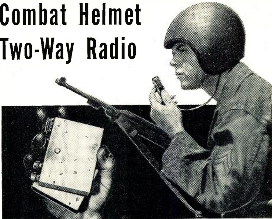
GI talks into a thumb-sized microphone that slips easily under his helmet when not in use. Inset shows the two small units that snap into a special plastic combat helmet. Top case holds the earphones, switches, and the 3 penlite-sized batteries used to operate the equipment. Lower case contains the transmitter and receiver circuits.
