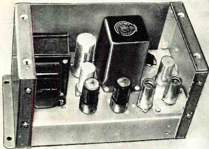
↑ Top view of the power amplifier with top and side panels removed. The audio output transformer can be clearly seen near the center of the chassis, while the power transformer is at the left. The four amplifier tubes, the electrolytic filter capacitors, and impedance selector switch are also visible on the chassis.
