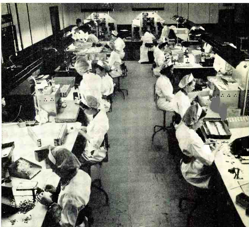
SEPARATE FACILITIES are maintained for the exclusive processing and manufacture of high reliability capacitors. Only specially trained, highly skilled operators, who wear special clothing to prevent any possible source contamination, work here.
