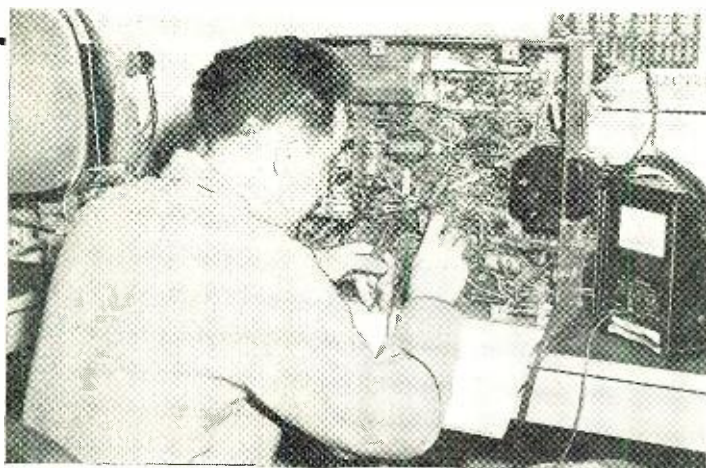
The only sure way to troubleshoot a receiver quickly and expertly is on the shop bench with test equipment and schematic diagrams.
