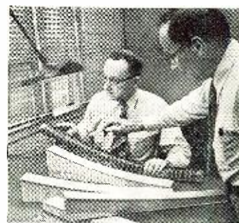
New type waveguide is bent on wooden forms for study of effect of curvature on transmission. The waveguide itself is here covered with a protective coating.
