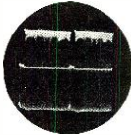
Fig. 2D. White compression due to a.g.c. fault.
