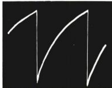
Fig. 3. Waveform at the grid of the horizontal output amplifier tube of a TV set; its amplitude is 40 to 60 volts.
