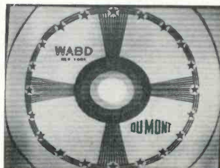
Fig. 5. Horizontal bar interference. Interference signals below 15,750 cps at the CRT cause this type of pattern.
