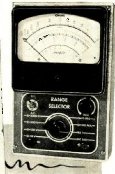
Two views of the meter panel on which all component parts are mounted.
