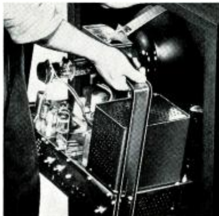
Fig. 2. The special chassis bracket on Stewart-Warner's TV sets makes removal from the cabinet very simple.
