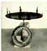
Light-weight (6 oz.), rugged, simple aperture mask of CBS-Colortron minimizes problems of exhaust, handling, and assembly.
