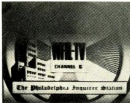
Fig. 1. Pattern produced on TV screen by 60-cycle hum interference in video.
