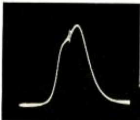
Fig. 4. The appearance of a beat marker or "birdie" on an i.f. response curve.
