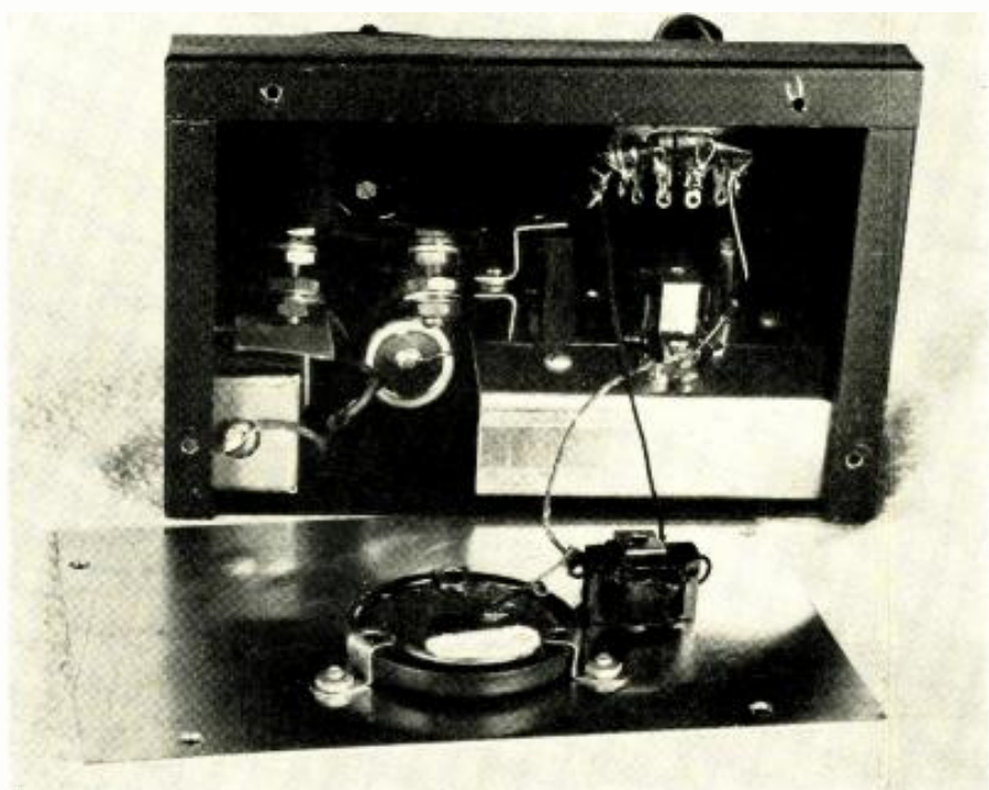
Fig. 3. Rear view of instrument. Microphone and transformer are mounted on the panel.
