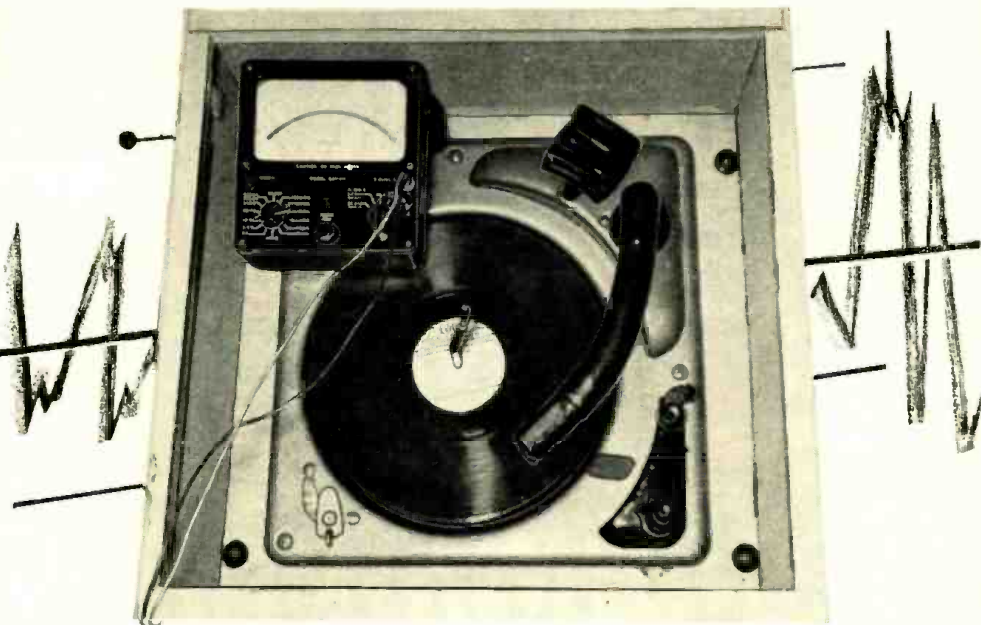
Fig. 1. Measuring the rhythm of turntable rumble to locate source.
