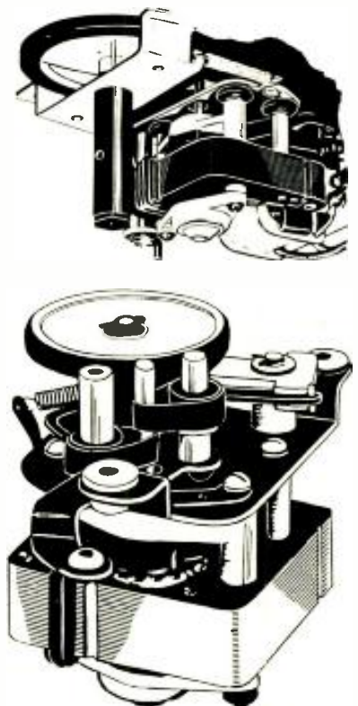
Fig. 6. Admiral and V-M speed reduction system using a set of pulleys with a belt drive from the motor armature shaft. →
