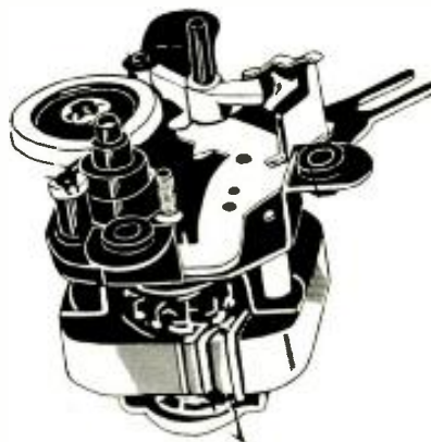
↑ Fig. 5. The Philco motor and speed reduction system uses a single drive shaft working against another shaft with three different size pulleys for various speeds.
