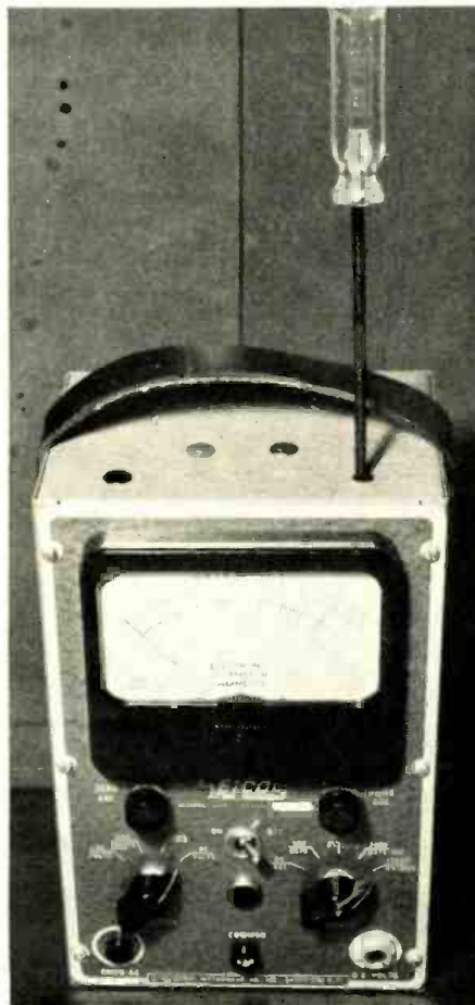
Template used to locate calibration holes in Eico Model 221 vacuum-tube voltmeter.
