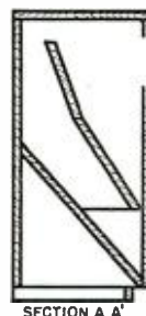
Fig. 5. Complete mechanical details for building "The Purist" enclosure. Care must be taken to insure an airtight seal otherwise performance will be impaired. All joints should be both screwed and glued for rigidity.
