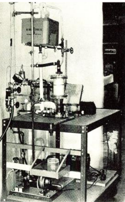
Fig. 2. Laboratory setup for use in ultrasonic depolymerization studies.
