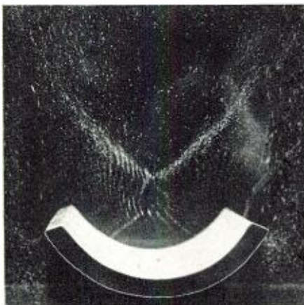
Fig. 8. A ceramic trough transducer immersed in a cleaning fluid.
